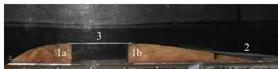
Fig. 39.13 Obstacle in Weinfurter et al. experiments (after [39.54]): (1a) and (1b) curved parts motivated by airplane wing; (2) flat aluminum plate to further reduce flow separation; and (3) flat top aluminum plate to reduce wave tunneling effects
