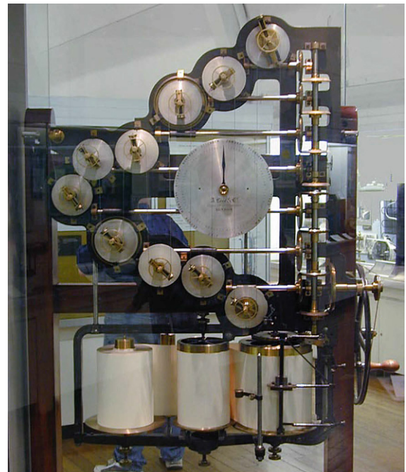
Fig. 31.3 Kelvin’s first tide predicting device (photo by William M. Connoley)
